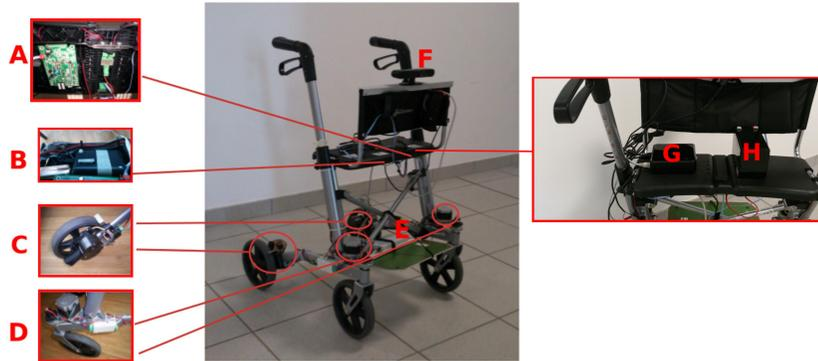
**Fig. 2** The *c-Walker* prototype along with its main components, i.e. the Beaglebone platform running low-level functions (A), IMU (B), encoders (C), motors (D), RFID Reader (E), Camera (e.g. Kinect) (F), the Barebone platform running high-level functions (G) and the main battery (H).
