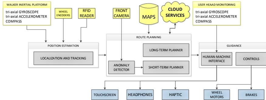
**Fig. 1** Functional block diagram of the *c-Walker*.
