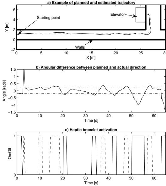
**Fig. 5** Planned route to the elevator (dashed line) and corresponding estimated path (solid line) (a). Difference between planned and measured direction angles along the way (b). Activation signals of the right (dashed line) and of the left (solid line) haptic bracelet (c).
